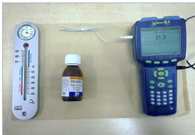
Fig.1: Sketch of measuring temperature inside nine types of drug bottles by thermocouple.
