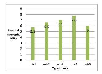
Figure (5) Flexural strength MPa at 28 days.
