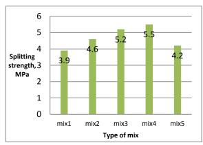
Figure (4) Splitting strength at 28 days.
