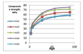
Figure (3) Compressive strength of different mixes.
