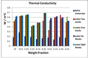
Fig. (7) Thermal conductivity of the samples as a function of weight fraction
