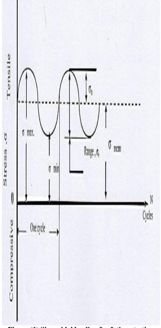
Figure (1) Sinusoidal loading for fatigue testing [17].
