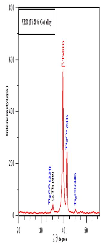
Fig.1: XRD patterns Ti-20%Co alloy uncoated.
