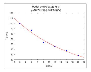
Figure (10) Example of (k) Estimation Using STATISTIC Software at Vg= 1cm/sec. and Cf=5 ppm of Caprlyic Acid
