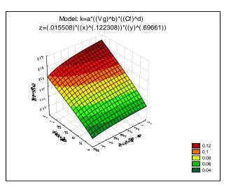
Figure (11) Relation of Kinetic Flotation Constant with Superfacial Gas Velocity and Frother concentration Using Caprylic Acid
