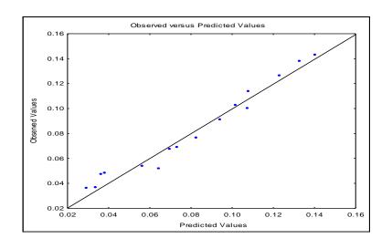
Figure (14) Relationship Between Predicted and Observed Value of Kinetic Constant Using Hexanol
