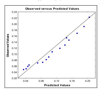
Figure (12) Relationship Between Predicted and Observed Value of Kinetic Constant Using Caprylic Acid
