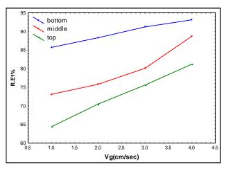
Figure (8) Effect of Gas Velocity on Removal Efficiency for Different Stage at Cf =15ppm of Hexanol
