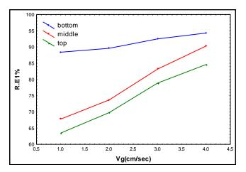
Figure (9) Effect of Gas Velocity on Removal Efficiency for Different Stage at Cf =20ppm of Hexanol
