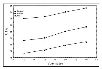
Figure (3) Effect of Gas Velocity on Removal Efficiency for Different Stage at Cf =10ppm of Caprylic acid
