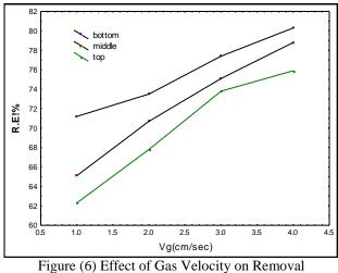
Efficiency for Different Stage at Cf =5ppm of Hexanol
