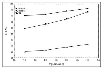
Figure (5) Effect of Gas Velocity on Removal Efficiency for Different Stage at Cf =20ppm of Caprylic acid
