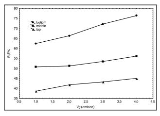
Figure (2) Effect of Gas Velocity on Removal Efficiency for Different Stage at Cf =5ppm of Caprylic acid
