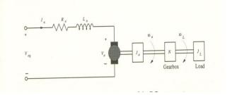
Fig.(1) DC motor circuit diagram
