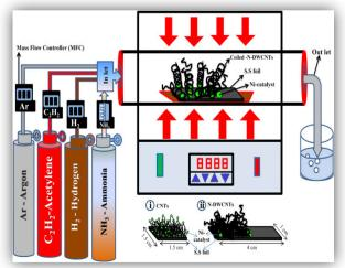
Fig.4:CVD method to produce MWCNT[15].
