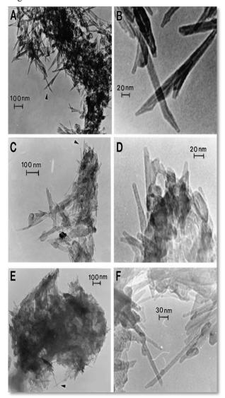
Fig.6: Natural Gas SEM. (A) a transmission electron microscope (TEM) a particulate matter (PM) sample. (B) High magnification of the area marked by the arrow in (A). (C) TEM snap of an environmental PM sample. (D) High magnification of the area marked by the arrow in (C). (E) TEM snap of an outdoor PM sample (F) High magnification of the area marked by the arrow in (E)[19].
