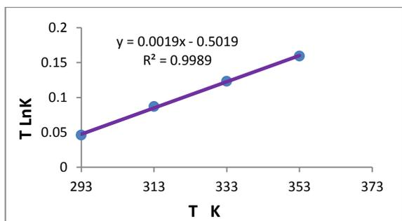
Fig. 12: Speed constant values for nickel ion capture mediated by poly(styrene-co- methyl metha acrylate) hydroxamic acid and at different temperatures.
