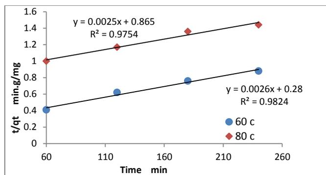
Fig. 11-b: Adsorption kinetics of nickel ion Ni<sup>2+</sup> mediated by poly(styrene-co-methyl metha acrylate) hydroxamic acid at temperatures 60 °C, 80 °C
