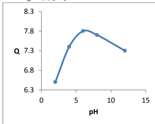
Fig. 9: Effect of the acidity function on the adsorption capacity of the nickel ion Ni<sup>2+</sup> by P.H.A
