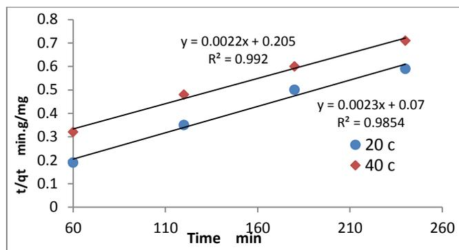
Fig. 11-a: Adsorption kinetics of nickel ion Ni<sup>2+</sup> mediated by poly(styrene-co-methyl metha acrylate) hydroxamic acid at temperatures 20 °C , 40 °C
