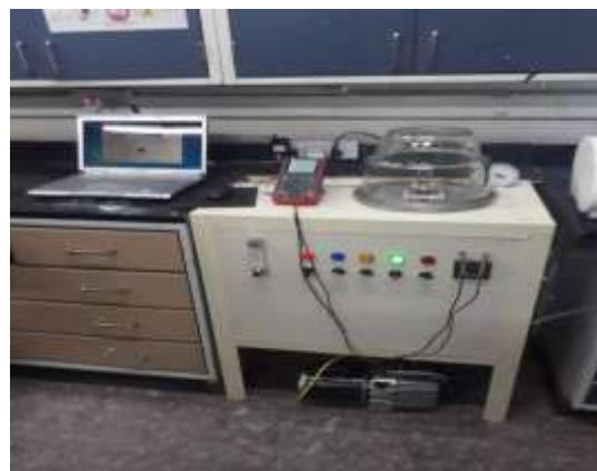
Fig. 1: Shows home-made gas sensing setup.
