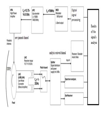
Figure 3.The block diagram for the jamming by the analysis of received signal<sup>[7]</sup>.
