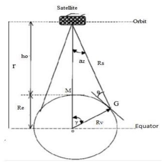
Figure 2. An illustration of coverage area and apex angle<sup>[3]</sup>.
