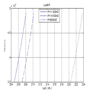
Figure 5.The relationship between path loss and traveled distance.
