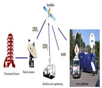
Figure 4.The method of jamming by using Satellite news gathering [8].
