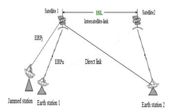
Figure 1. Dimensional distance between satellite and fixed earth stations<sup>[1]</sup>.
