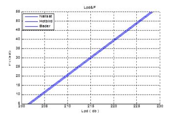
Figure 6. The relationship between the path loss factor and frequency of the up-link distance for satellites (Nile sat, Hot bird, Bader).
