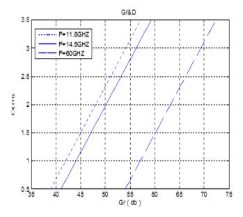
Figure 7. The relationship between antenna's diameter and gain of different frequencies .
