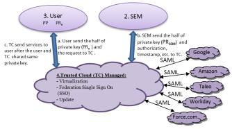
Figure 9. Lower part of proposed system architecture
