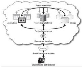
Figure 1.Cloud computing according to NIST definition [1]
