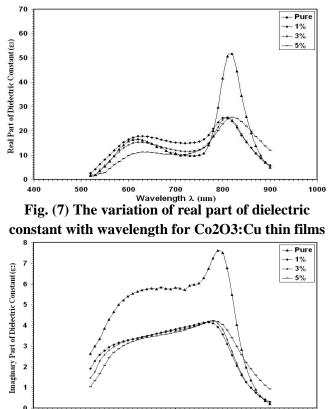
Wavelength λ (nm) Fig. (8) The variation of imaginary part of dielectric constant with wavelength for Co2O3:Cu thin films
