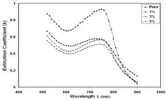
Fig. (6) The variation of extinction coefficient with wavelength for Co2O3:Cu thin films.
