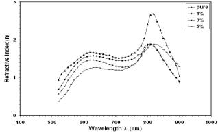
Fig. (5) The variation of refractive index with wavelength for Co2O3:Cu thin films.
