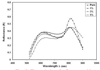
Fig. (2) The variation of reflectance with wavelength for Co2O3:Cu thin films.
