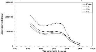
Fig. (3) The variation of Absorption coefficient with wavelength for Co2O3:Cu thin films.
